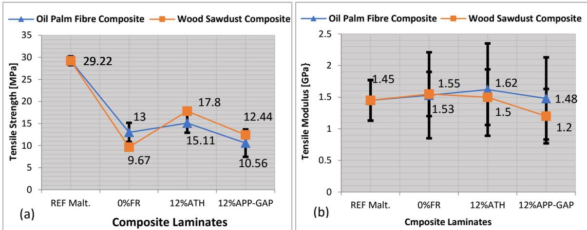
Figure 2: Composite laminates at 12% FR loading (a) Tensile strength (b) Tensile modulus
