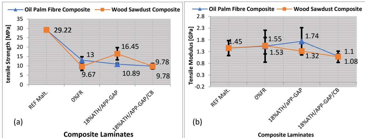
Figure 4: Composite laminates at 18% FR loading (a) Tensile strength (b) Tensile modulus
