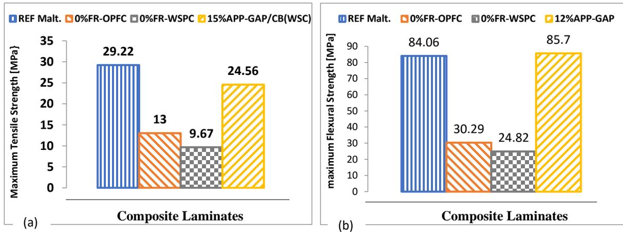
Figure 6: Comparison of the maximum composite laminate (a) tensile strength (b) Flexural strength with the reference material and those without FR
