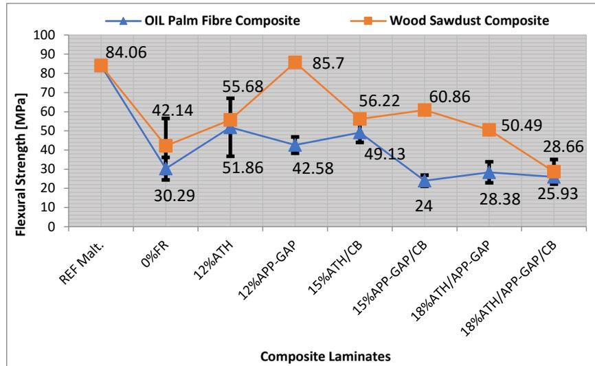
Figure 5: Flexural strength for the composite laminates at various FR loading
