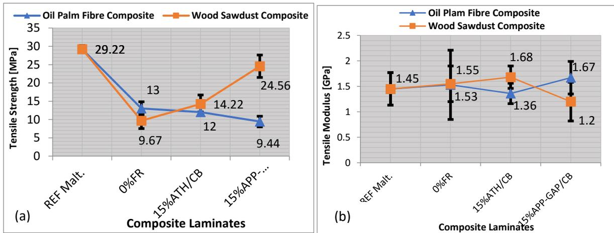
Figure 3: Composite laminates at 15% FR loading (a) Tensile strength (b) Tensile modulus
