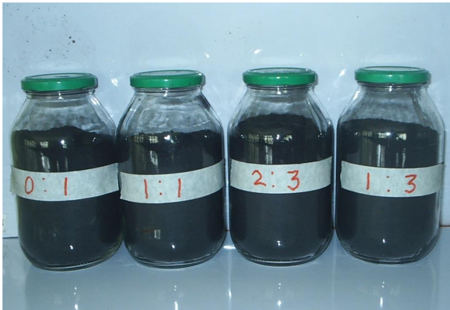
Plate 1: Cassava Peel Carbon (CPC) and Cassava Peel Activated Carbon (CPAC) materials stored in jars
