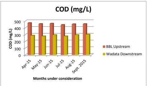
Fig. 4Plot of the Chemical Oxygen Demand for the water samplesFig. 5Plot of the Hardness Test for the water samples
